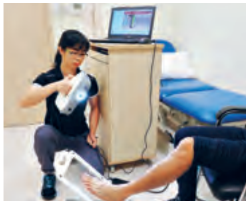
LEFT The TTSH Foot Care and Limb Design Centre uses handheld scanners and 3D software to create customised ankle-foot orthotic braces.
